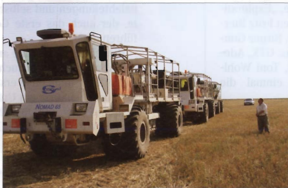
Three vibrator trucks produced the seismic energy to penetrate the rock. Foto: Wintershall
